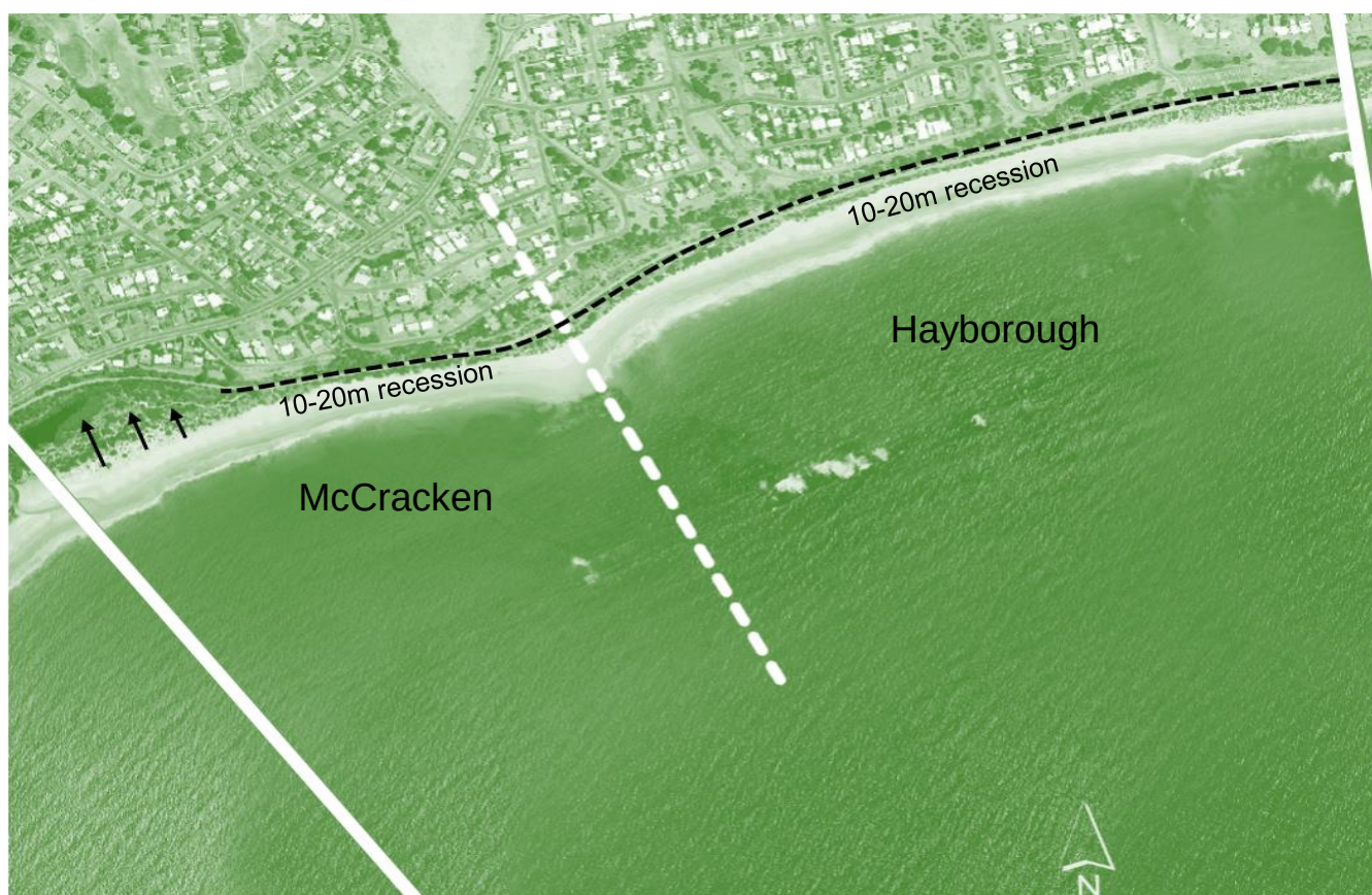
Figure 3. The extent of shoreline recession anticipated for 2050 to 2100, which would significantly impact the dunes and embankment under the trainline.
