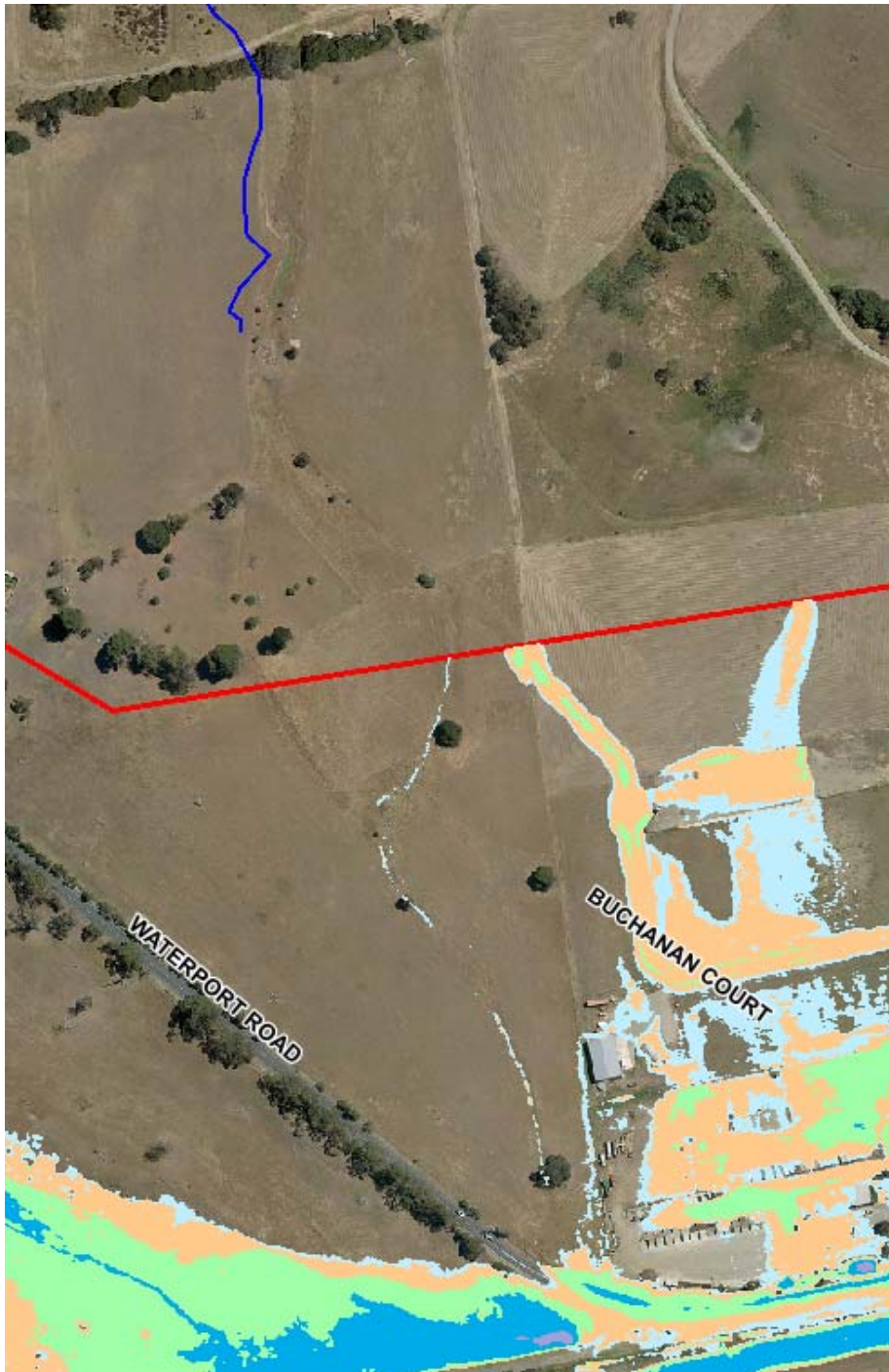
Figure 6.1 Watercourse with Split in Flow Path (1% AEP)
