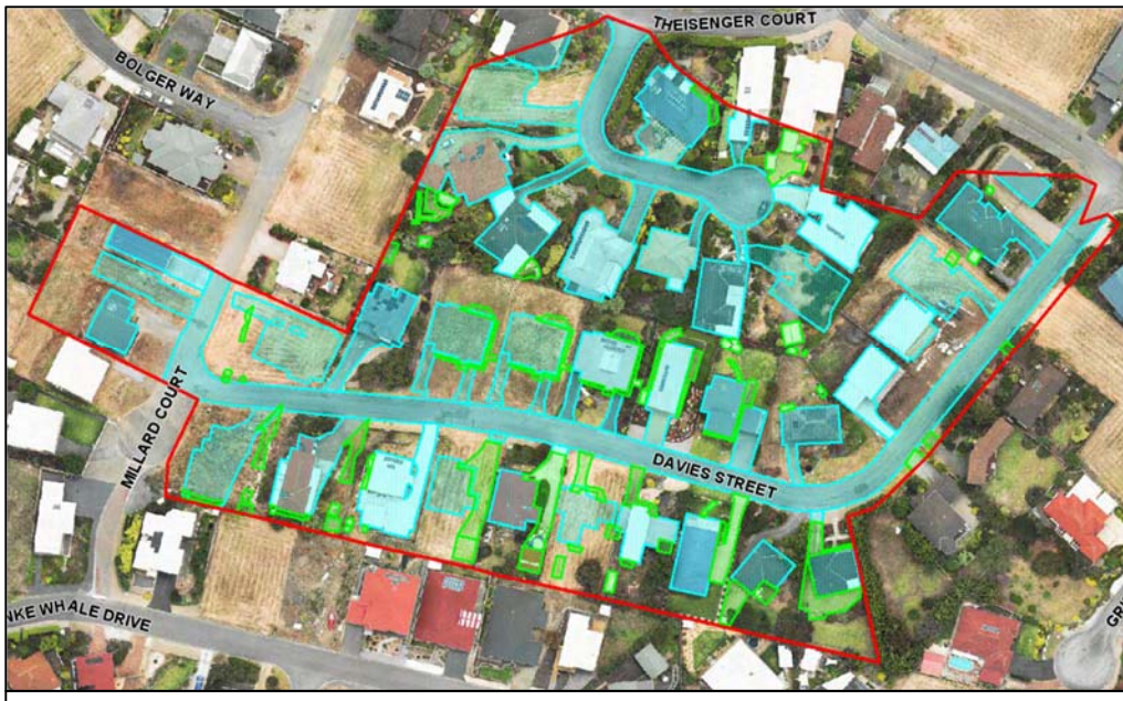
Figure 3.6 Impervious Fraction, Davies St Sub-Area
